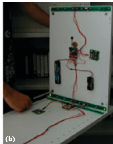
2 LED lights on the components guide the user in the assembly process: (a) rotation and (b) screwing.
